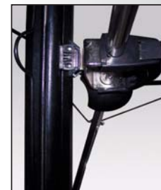
Case welded to handle
